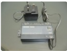
Kramer 482 Bi-directional audio transcoder (balanced/unbalanced) with gain controls and PSU
