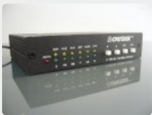
Lot: 802 TV One 1T-TBC-GL Ultra compact time base corrector with genlock. Includes PSU.
