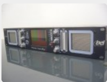
Lot: 772 Bel AV2 Broadcast monitoring unit SDI/AES with TFT screen, bargraph metering, speakers
