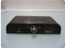
Lot: 713 HD/SD-SDI to HDMI converter (auto-detects input). All resolutions up to 1080p
