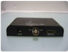
HD/SD-SDI to HDMI converter (auto-detects input). All resolutions up to 1080p
