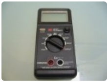
Caltex CM3230 Digital capacitance meter (200pF to 20000uF ranges)
