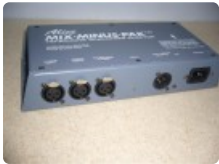
Lot: 173 Alice Mix-Minus-Pak - generates clean feed from mixer output minus the telephone
