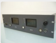
Lot: 154 PPM unit: AES/EBU Digital input twin stereo with bit rate indicators and analogue outputs
