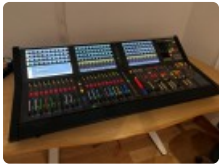
Lot: 251 Studer Vista 1 Black Edition Broadcast, Live and Production Mixing System 32 motorised faders [VISTA 1 BLK 32F] Dual Madi I/O Card D23m installed.
