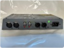
Lot: 852 Alice Broadcast Match Pak 4ch bi direction WITH GAINS balanced unbalanced balanced 2ch each way all ch tested OK
