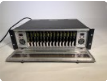
Evertz 7700FC-C Multiframe C10 with 1x 7700FC Control Card and 8x 7707CVTA35-2 and 6x 7707CVT35-2 cards
