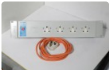
Lot: 497 Olson 2U rewirable 4-output 13A 19in rack mount power distribution; end mounting plates can be reversed (socket inside or outside rack) , External Earth point.
