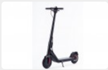
Lot: 146 E-Scooter NEW/BOXED: Max speed: 25km/h. 8.5in tyres, Torque: 16NM. Motor : 250W. Max instantaneous power: 500W. Max incline: Approx 15-18°. FOC control system + Cruise control. Travel Distance: 28km. Disk braking & eABS regenerative braking. Headlights: 15W ultra-bright headlights, 5m range. LCD Display. Max Load: 120KG
