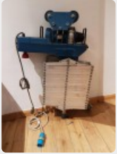
Lot: 631 Berkey Colortran MOTORISED lighting pantograph [max 37kg load]
