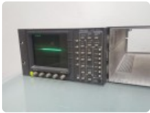
Lot: 767 Tektronix WFM1765 Stereo audio + component video waveform monitor: NTSC/PAL with Vector, Lightning, Diamond & Bowtie displays with 9 memories
