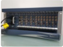
Lot: 481 Thomson Vibe AA Encoder with SP ENC (SDI) cards [x3], AA ENC (Analogue audio) cards [x3], CORE DEC (SDI / Digital audio) cards [x4] and AAV DEC (CVS & Analogue audio) cards [x 4]
