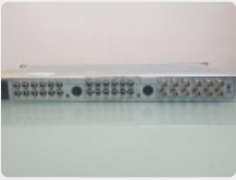
Lot: 550 MW Video DVA10: 10 video & 10 audio outputs, 1 video input & 2 audio inputs
