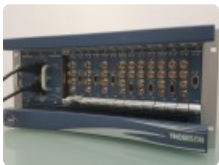
Lot: 413 Thomson Vibe AA Encoder with SP ENC (SDI) cards [x4], AA ENC (Analogue audio) cards [x4], CORE DEC (SDI / Digital audio) cards [x3] and AAV DEC (CVS & Analogue audio) cards [x 3]
