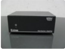
Lot: 642 Extron MDA 3AV one input, three output composite video with stereo audio distribution amplifier
