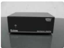
Lot: 791 Extron MDA 3AV one input, three output composite video with stereo audio distribution amplifier
