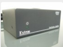
Lot: 726 VersaTools MDA-3AV 1-into-3 Video and stereo audio distribution with PSU
